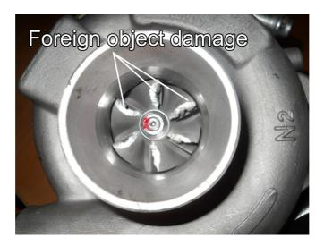
Check the old nut if it has not been left in the intercooler, because it will destroy each subsequent turbine when there is no lubrication, i.e. the oil supply tube is clogged by thick oil or dirt or the oil pump tube is clogged or the pump stops draining the oil or oil pressure, the turbine shaft will be overheated and destroyed the oil bearings will not be accepted warranty for the turbine.
