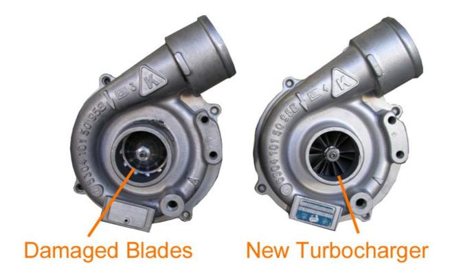
The left turbocharger has been damaged by some foreign object that has entered the system. Compared to the turbocharger on the right, which is new, the damage is clearly visible. Foreign body damage will void the parts warranty. See the image below for a close-up of the foreign body injury.
